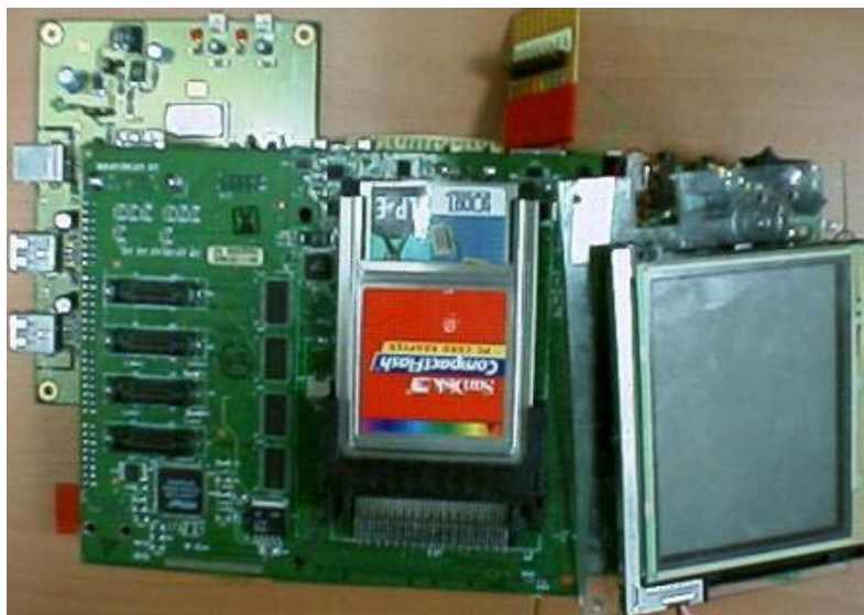
Figure A-4: ISPI I60x Evaluation, StrongBridge, StrongARM Development Kit and StrongARM Companion Chip Development Kit
